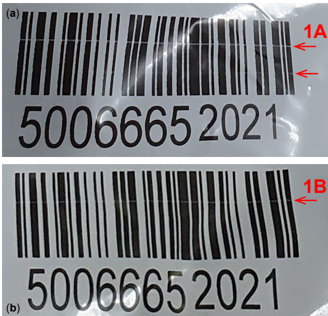
FIG. 15. Barcodes on both bags were printed by the same thermal transfer printer, as evidenced by the same position of a prominent dead-pixel white line. (a) Bag A. (b) Bag B. The second faint line is not visible owing to a lower resolution of the latter image.
