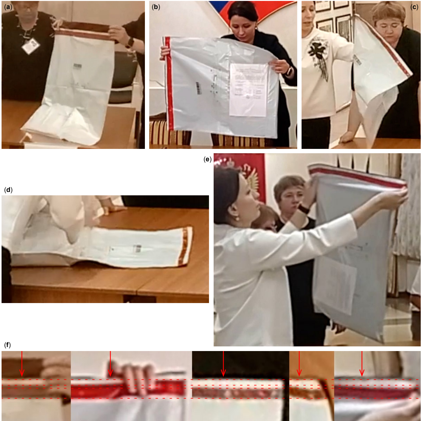
FIG. 26. Frames from video recordings of the second security bag at precinct 214 after sealing the bag on the second day made by (a) camera 1 and (b) camera 2, then before opening this bag during the vote counting on the third day made by (c) camera 1, (d) camera 1, and (e) camera 2. (f) A collage between rotated fragments of (a)–(e) shows the changed tape width and distance from the edge, as well as consistency of our geometry estimation between different cameras and viewing angles. The arrow denotes a point about 1/4 the bag width from its right edge in each collage segment. The tape width can also be compared to the height of the barcode visible in the images, which is 20 mm, according to the factory specification [57]. Using that as a reference, the tape width in images (a) and (b) measures no less than 30 mm, while it is close to 20 mm in images (c) and (d).
