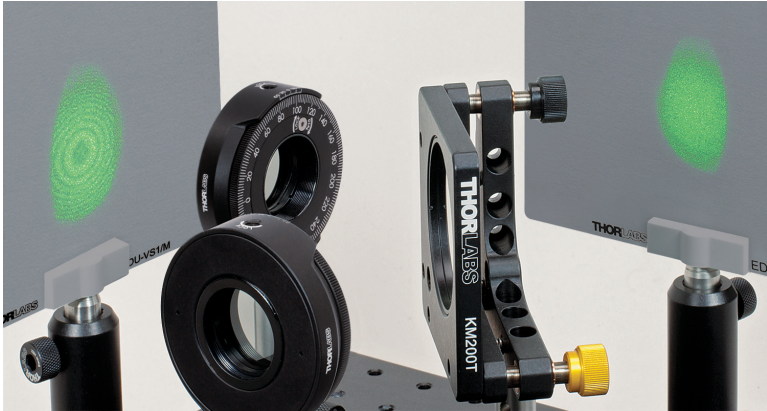
Figure 14 Right Screen: No Interference Pattern. Left Screen: Interference Pattern Behind the Eraser
